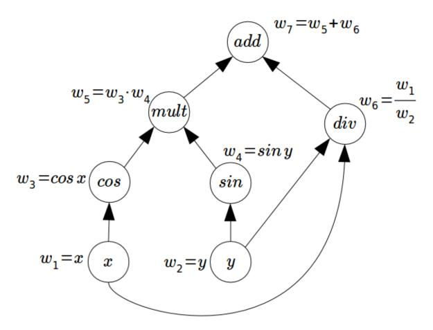
In the example above, the w1 node contains the gradient for input x at some value, the data from w1 is then passed through the cos() operation to create w3. w3 is later multiplied with w4 to create w5, and so on. We will pass our input value along the "trace", and by judicious application of the chain rule, we will compute the derivative of the overall function. The traces can be through of as the ordered set of operations that the data undergoes.
