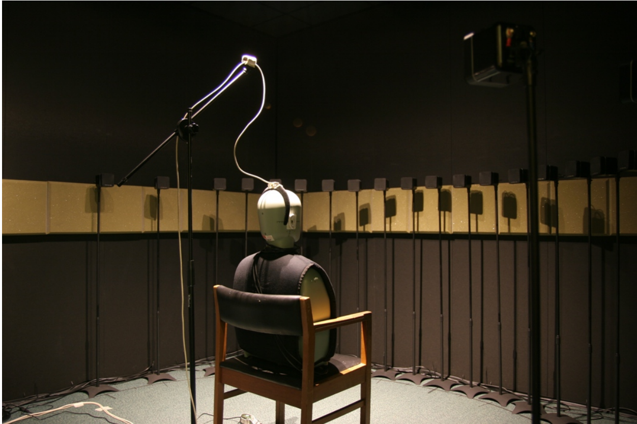
Fig. 3.3: Photo of the laboratory with a dummy head instead of a participant.
