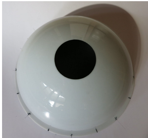
Fig. 9: Second set of marks spaced at 45 degrees, located between first set of marks
