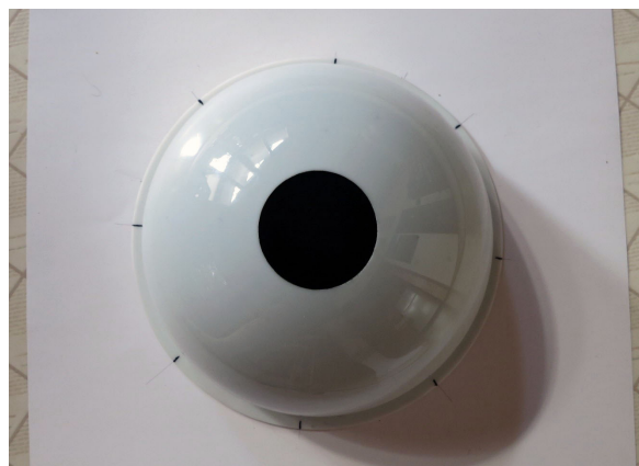
Fig. 8: Dome flange marked at 45-degree increments
