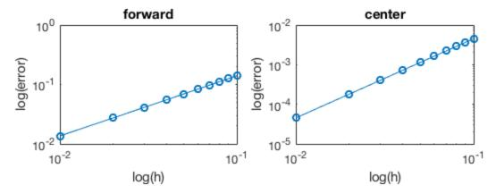
To figure out the slope we can do linear regression. You can solve a least square problem as in HW4&5, but here we use a shortcut as described in this example. polyfit(x, y, 1) returns the slope and intercept.
