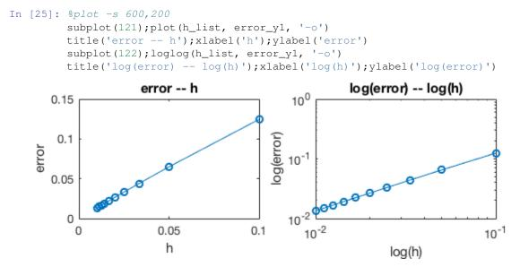
Of course we can still calculate the slope of the log-log plot, to double check the forward Euler scheme is a first-order method.
