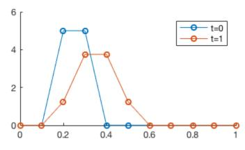
We got a pretty huge error here. After  $t = 0.5 \times 2 = 1$ , the solution should just be shifted by one grid point, like in the previous naive PDE "solver". Here the center of the chemical field seems alright (changed from 0.25 to 0.35), but the chemical gets diffused pretty badly. That's due to the numerical error of the first-order scheme.
