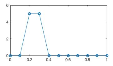
Say the chemical is blew by the wind towards the right. At the next time step the field is **shifted rightward by 1 grid point**.
