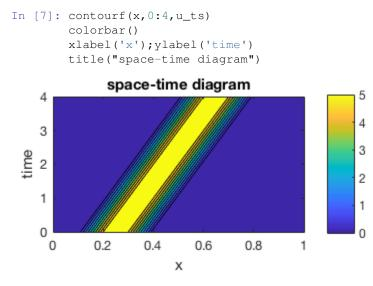
Here we can clearly see the "chemical field" is moving rightward through time.
