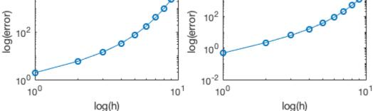
Now the error is super large and the log-log plot is not a straight line. So keep in mind that for most numerical schemes we always assume small h.
