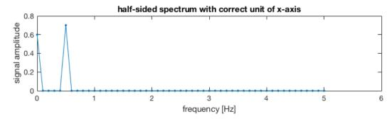
The peak is at 0.5 Hz, consistent with our original signal which has a period of 2 s, since 0.5 Hz = 1/(2s). Thus our unit specification is correct.
