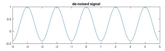
The de-noised signal is almost the same as the original noise-free signal:
