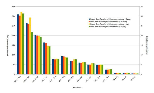
From the picture above, we can discover that as frame size decreases, data throughput also decreases, rapidly. So in our later experiments, we should use a relatively small frame size to obtain low data throughput, so that our system doesn't need to handle high pressure of data.
