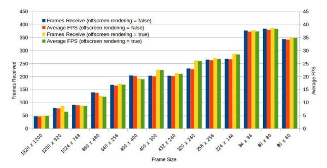
In general, as can be seen, as frame size decreases, we will have higher FPS and receive more frames. So in our future experiments, we should use a relatively small frame size to obtain high FPS, so that the game runs smoothly. And in most cases, turning on the offscreen rendering option will result in higher FPS.
