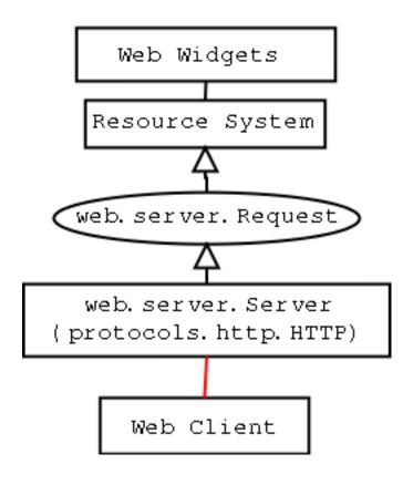
When the Web Server receives a request from a Client, it creates a Request object and passes it on to the Resource system. The Resource system dispatches to the appropriate Resource object based on what path was requested by the client. The Resource is asked to render itself, and the result is returned to the client.
