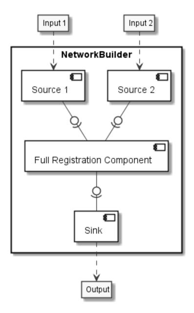
Fig. 2: Components can fulfill many tasks upto a full registration pipeline.
