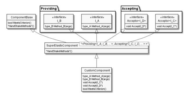
Fig. 1: UML class inheritance diagram of a Component in SuperElastix
