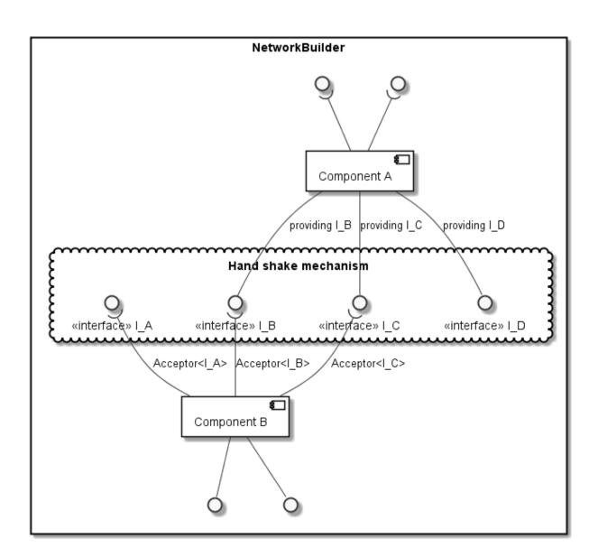
Fig. 3: The handshake mechanism validates whether components can be connected or not.
