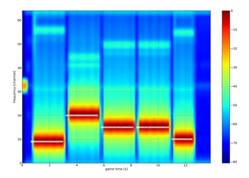
Similar to the upper graph in the per-player visualization, this graph shows a time-frequency diagram. The color on the diagram shows signal level, as reported by the actual spectrum sensor, for each channel and moment in time while the game was running.
