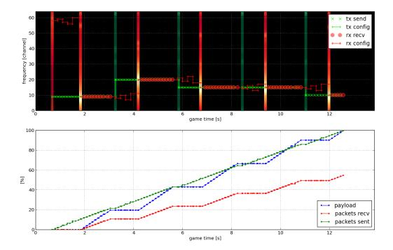
The upper graph with the black background shows the progress of the game in a time-frequency diagram. Game time is on the horizontal axis and frequency channels are on the vertical. Key events in the game are displayed in this diagram with the focus on the current player.
