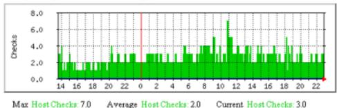
A good way to determine the proper value for the cached check horizon options is to compare how many on-demand checks Shinken has to actually run versus how may it can use cached values for. The *nagiostats* utility can produce information on cached checks, which can then be *graphed with MRTG*. Example MRTG graphs that show cached vs. actual on-demand checks are shown to the right.
