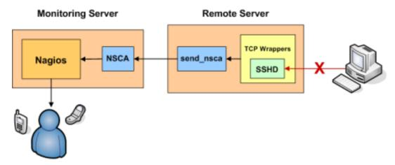
This document explains how to easily generate alerts in Shinken for connection attempts that are rejected by TCP wrappers. For example, if an unauthorized host attempts to connect to your "SSH" server, you can receive an alert in Shinken that contains the name of the host that was rejected. If you implement this on your Linux/Unix boxes, you'll be surprised how many port scans you can detect across your network.
