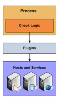
Active checks are initiated by the check logic in the Shinken daemon. When Shinken needs to check the status of a host or service it will execute a plugin and pass it information about what needs to be checked. The plugin will then check the operational state of the host or service and report the results back to the Shinken daemon. Shinken will process the results of the host or service check and take appropriate action as necessary (e.g. send notifications, run event handlers, etc).
