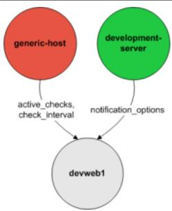
In the example above, devweb1 is inheriting variables/values from two sources: generic-host and development-server. You'll notice that a check\_interval variable is defined in both sources. Since generic-host was the first template specified in devweb1's use directive, its value for the "check\_interval" variable is inherited by the devweb1 host. After inheritance, the effective definition of devweb1 would be as follows:
