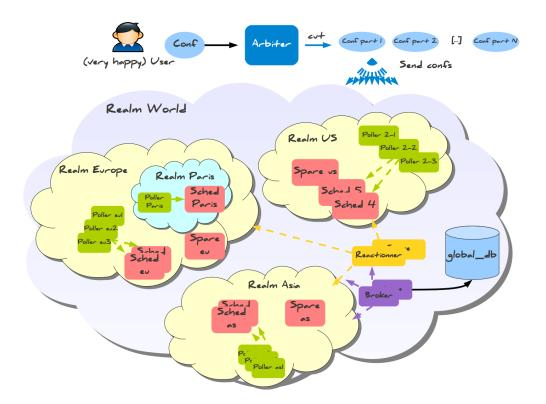
Satellites can be used for their realm or sub realms too. It's just a parameter in the configuration of the element.
