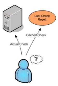
The performance of Shinken's monitoring logic can be significantly improved by implementing the use of cached checks. Cached checks allow Shinken to forgo executing a host or service check command if it determines a relatively recent check result will do instead.
