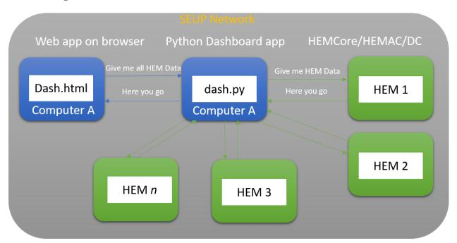
The app dash.py runs on a computer which is on the same network (local or through VPN) as HEM. It pulls data from all these HEMs and also has the capability to send actuation signals to all the HEMs. Usually, the HEMs are all assigned static IPs and these are pre-defined and known to all applications.
