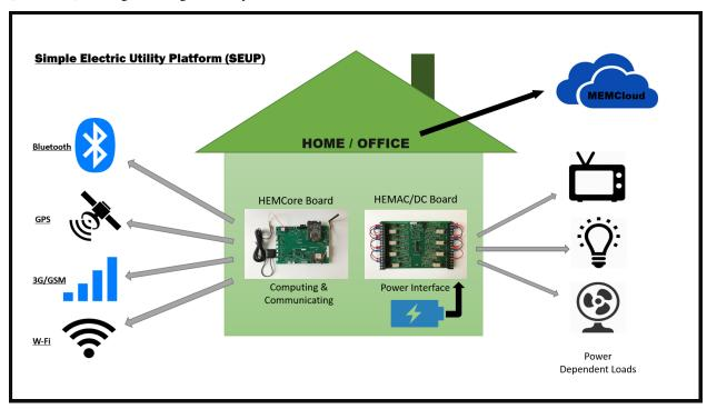
The system comes with a variety of communication features including: cellular, Wireless/Wired and Bluetooth. This not only allows for more flexibility in how one can control their grid but it also provides the user with a backup in case one feature cannot be accessed at a given time. The grid uses the cloud for encrypted data transmission/reception meaning your information is protected. GPS functionality allows users to geolocate their grid to get accurate scheduling time
