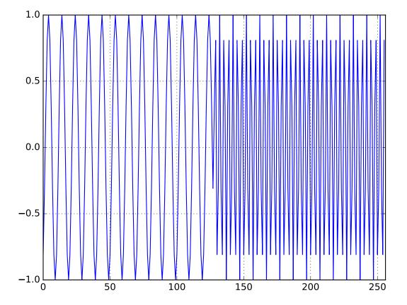
This first half of the signal is a sinusoid with a normalized frequency of 0.1 and the other half has a normalized frequency of 0.3. If we look at the energy spectrum of this signal, sure enough, there are two peaks at the respective frequencies:
