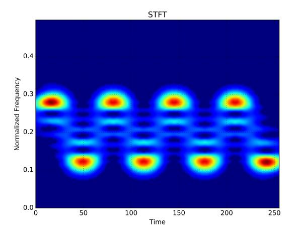
From this representation, the sinusoidal nature of the frequencies can be made out, and even the concentration of energy at the extrema of the sine wave makes sense. But the artifacts between the high energy areas are quite ambiguous, and bear little resemblance to the signal's true characterisites.
