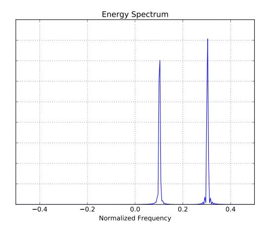
Note that the signal produced by the fmconst function produces an Analytic Signal. Analytic signals are complex valued, and by definition do not have negative frequency components.
