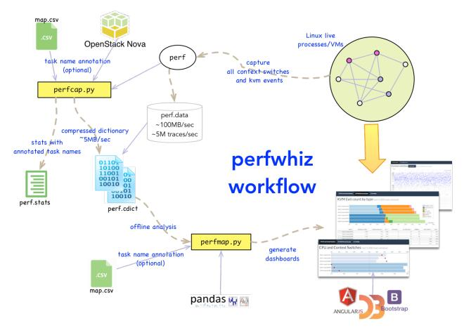
Capture is performed on the system under test, by invoking the perfcap.py script and specify which tasks to capture events from and for how long. The result of each capture is a binary file (with the cdict extension, cdict stands for compressed dictionary).
