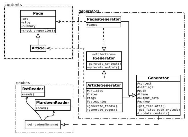
The interface does not really exist, and I have added it only to clarify the whole picture. I do use duck typing and not interfaces.
