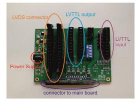
The breakout board provides the connectors for the various Bus systems. The LVTTL inouts and outputs are connected to the digital input and output cards, which provide a galvanic isolation. The LVDS bus is connected to the DDS devices that provide an analog RF output.
