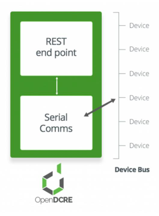
The OpenDCRE device bus is comprised of a set of boards and devices, individually addressable, and globally scannable for a real-time inventory of addressable devices attached to the bus. The OpenDCRE device bus allows devices to be read and written, and for various actions to be carried out, such as power control (on/off/cycle/status). Additionally, when a physical OpenDCRE device bus is not present, a software emulator can be used to simulate OpenDCRE API commands and functionality.
