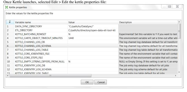
Right-click to insert a new line. Once a blank line is available, add ETL\_DIRECTORY as a variable name and add the path to your ETL directory under value (e.g., C:/path/to/directory/open-data-utility-kit).
