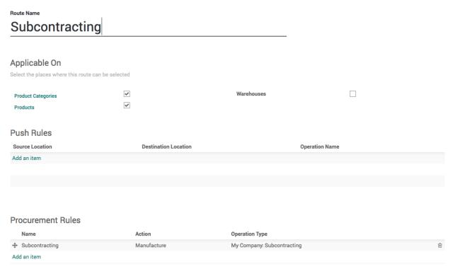
Create a procurement rules that applied on WH/Stock location and ask WH/Contractor location to fulfil by creating a manufacturing order. This configuration will create the manufacturing order at Contractor location and looking for the
