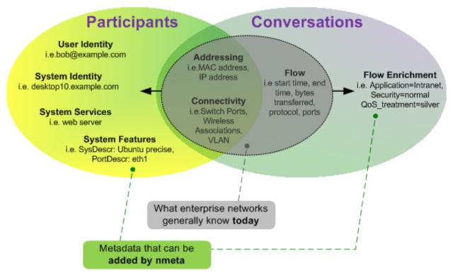
The goal of the nmeta project is to produce network metadata enriched with participant identities and conversation types to provide a foundation for innovation in networking.
