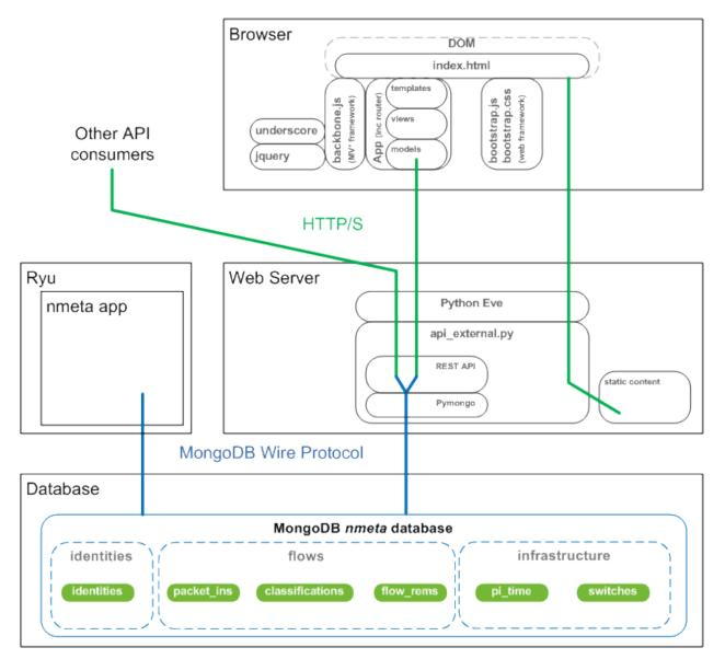
The Web Server, Ryu/nmeta and the MongoDB database all run independently. Backbone.js is the JavaScript framework used to power the UI in the browser. Bootstrap is the web framework used to style the presentation of the UI.
