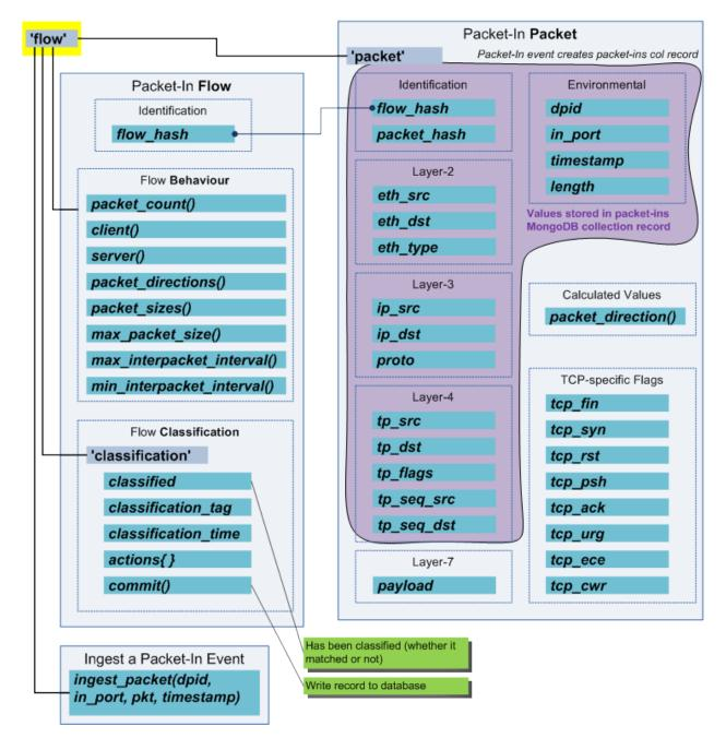
Classifiers can make use of the flows object to gain easy access to features of the current flow.
