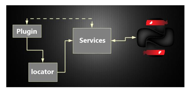
The image above shows the connection between plugins and NINJA-IDE. Plugins get services by using a service locator. The service locator returns the specific service and the plugin uses this service to talk with NINJA-IDE.
