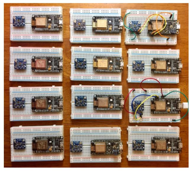
I verified that each board was functional by flashing the latest version of MicroPython to it. I did not test the light sensors, but did have a spare.
