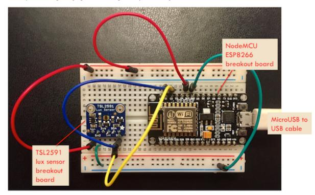
And, finally, here is a photograph of the completed system using the NodeMCU board:
