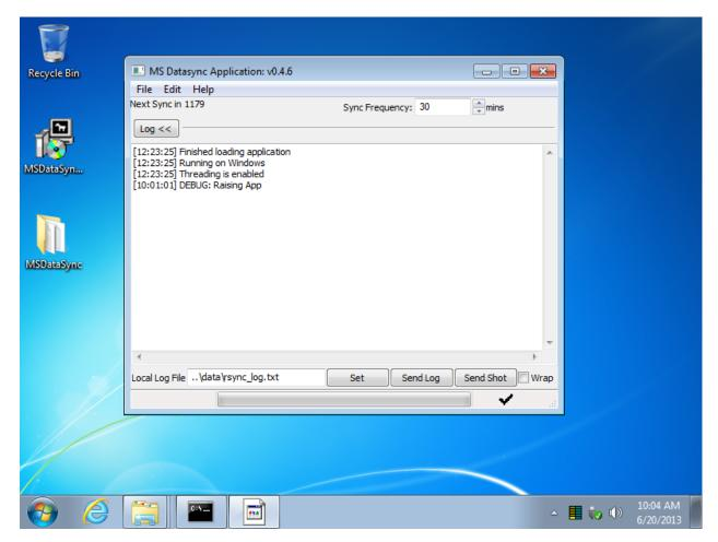
The Mastr-MS data sync client should be installed on the Windows machine which is connected to the lab instrument.
