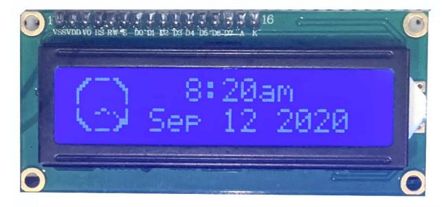
It is a very popular LCD display that is widely available, cheap and available in several form factors with 16 character x 2 line and 20 character by 4 line displays the most common. As with most LCD displays, it comes with a backlight which luma.lcd can control using a GPIO pin. PWM modulation is supported if varying the intensity of the backlight is desired.
