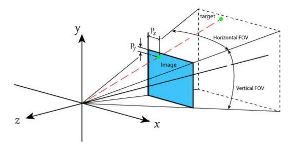
Our first step will be to convert from pixel coordinates to normalized 2D coordinates where 0,0 is the center of the image and 1.0:
