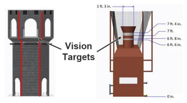
These retro-reflective vision targets have a very useful property: when light is shined at them, it will reflect directly back to the light source. This is why Limelight has bright green LEDs surrounding its camera lens. By setting the camera exposure very low while emitting a bright green light toward the target, we can acquire an image that is mostly black with a bright green vision target. This makes the job of acquiring the target relatively easy.
