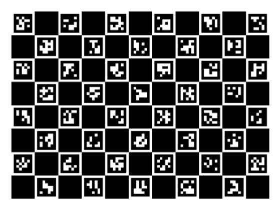
www.calib.io | 8x11 | Checker Size: 15 mm | Marker Size: 12 mm | Dictionary: AruCo DICT\_5X5.
