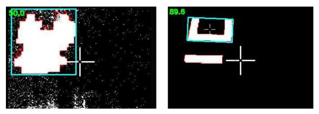
Sometimes things like ceiling lights or windows in an arena can be difficult to remove from the image using thresholding, which brings us to the next stage.
