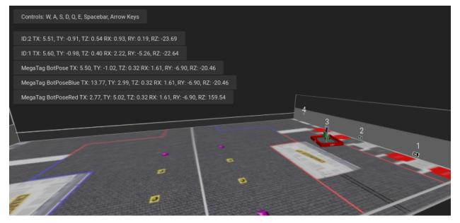
All botposes are printed directly in the field-space visualizer in the web interface, making it easy to confirm at a glance that everything is working properly.
