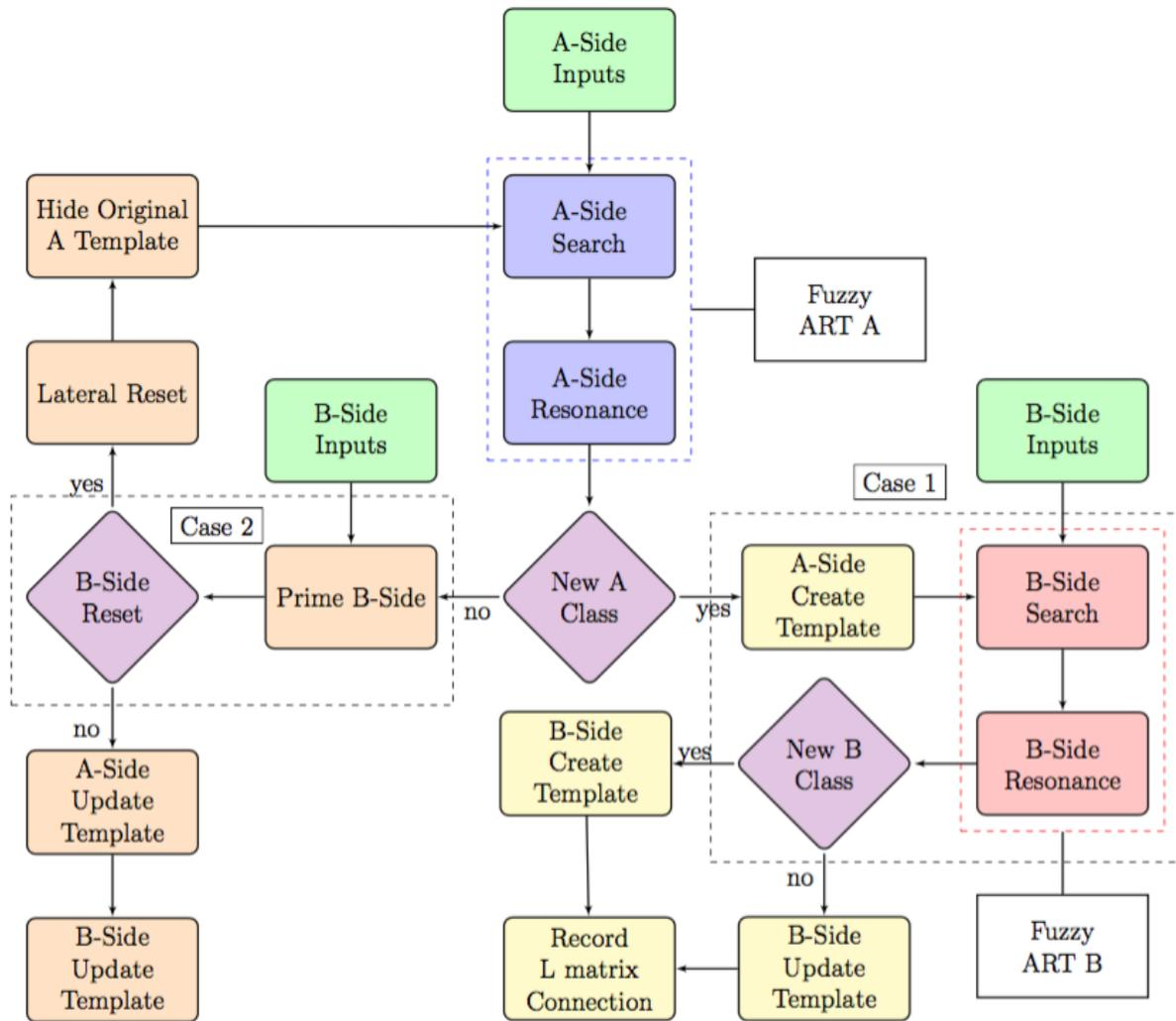
Figure 1.1: LAPART training algorithm flow diagram includes Fuzzy ART A & B and two cases for learning A and B side templates.
