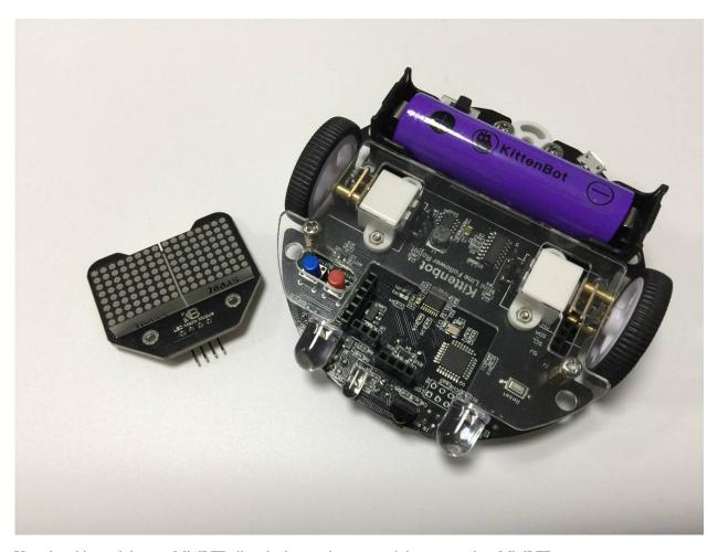
You plug this module onto MiniLFR directly, just as the two modules mounted on MiniLFR.
