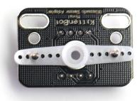
Insert the assembled parts on the servo rotor and tighten it with the small screws from the servo part package.
