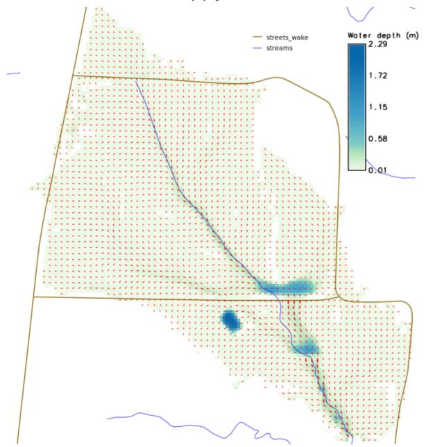
One option to solve this problem is to model a culvert using the coupled modelling capacity of Itzï. Itzï is able to run the SWMM drainage model alongside the surface model, and model the interactions between the two.
