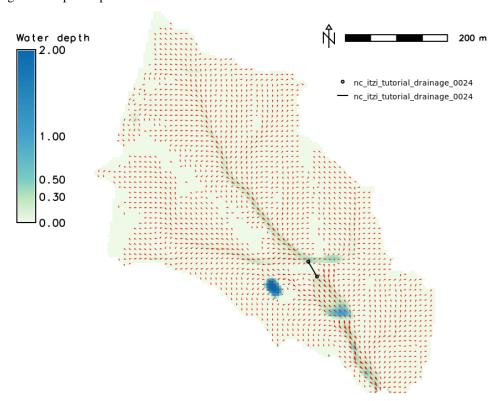
The area upstream the road is noticeably less flooded, with a maximum water depth coming down from 1.03m without culvert to 0.45m with culvert. You can use the temporal tools of GRASS to query the evolution in time of the drainage network values. For example, to get the evolution of the flow leaving the upstream node *J0* of the culvert:
