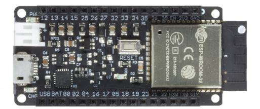
Very small and breadboard-friendly with option of male, female or both (stackable headers). Includes a dual-core 240 MHz ESP32 with WiFi and Bluetooth. You can use the WiFi both in station (device) mode and access point mode. It includes traditional Bluetooth as well as BLE 4.0.
