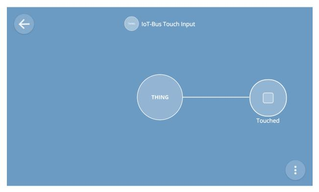
The onboard LED will light when the wire is touched and turn off when the wire is released. At the same time the Mozilla IoT interface will reflect the status of the wire whether touched or not. There are lots more examples in PlatformIO format here or in Arduino format.
