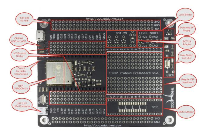
The board includes a large prototyping area that includes room for traditional DIP and through-hole components as well as SMD parts such as SOIC and SOT-23. A user LED and switch is included but not connected to any pins so you can use them how you wish. Two level shifters are included so you can interface with 5V devices.
