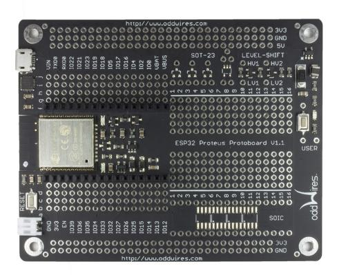
This board is larger and designed to make it possible to add your own circuitry to make a complete IoT solution on one board. It includes a dual-core 240 MHz ESP32 with WiFi and Bluetooth. You can use the WiFi both in station (device) mode and access point mode. It includes traditional Bluetooth as well as BLE 4.0. On-board is a 3.3V regulator and a battery charging device that enables you to switch between using USB or battery power.
