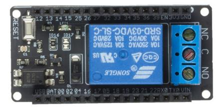
This is an opto-isolated relay board driven by a single digital pin. It is a 110V, 10A maximum AC relay board in the IoT-Bus form factor.
