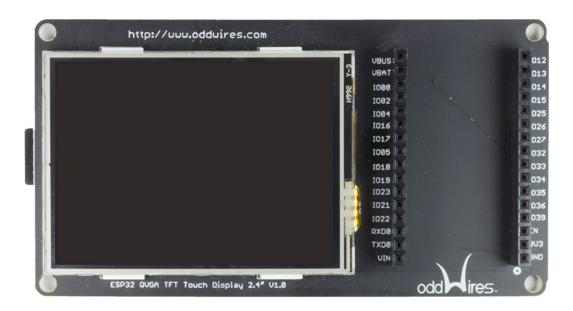
This a nice 2.4" 320x240 QVGA TFT Touch Display offering plug and play display output and touch sensing together with a 4-bit SDMMC SD Card. We picked 2.4" over 2.8" as it has a crisper display at 320 x 240 resolution and its slightly smaller size helps in IoT applications. Designed primarily for development use it has an IoT-Bus socket at the side for easy access. Here's the back view:
