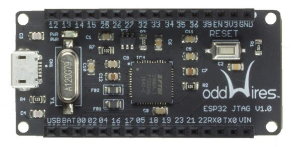
This IoT-Bus module provides JTAG debugging for the *Io* and *Proteus* boards (can be used with other boards too, see wiring connections below).
