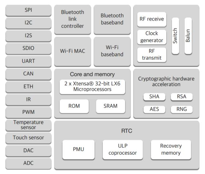
The ESP-WROOM-32 WiFi Bluetooth combo module is ultra high performance and ultra low-power consumption FCC-approved (2AC7Z-ESPWROOM32) Wi-Fi and Bluetooth combo wireless platform based on ESPRESSIF ESP32 chipset. It integrates a dual-core processor, 448 KByte ROM,520 KByte SRAM,16 KByte SRAM in RTC, 802.11 b/g/n/e/I Wi-Fi, Bluetooth v4.2 BR/EDR & BLE, clocks & Times, abundant peripheral Interfaces and security mechanism.
