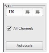
Gain can be adjusted for a single channel or, with the All Channels checkbox selected, for every channel on the headstage. The autoscale button will try to calculate the optimal gain value for the channel which is displayed.
