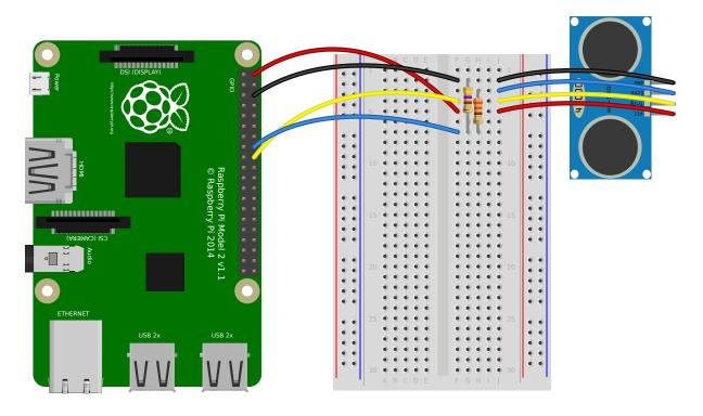
**Note:** In the diagram above, the wires leading from the sensor to the breadboard can be omitted; simply plug the sensor directly into the breadboard facing the edge (unfortunately this is difficult to illustrate in the diagram without the sensor's diagram obscuring most of the breadboard!)
