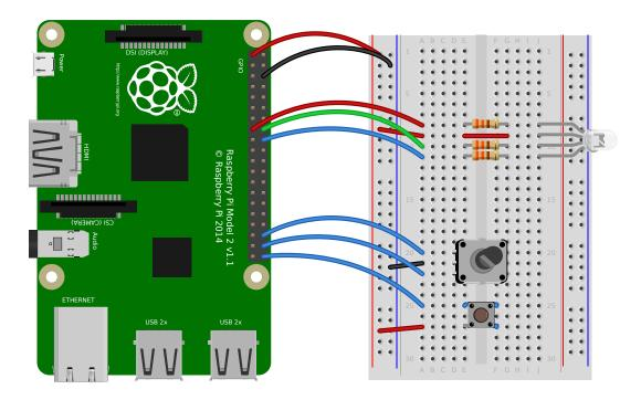
**Note:** In this recipe, I've used a common *anode* RGB LED. Often, Pi projects use common *cathode* RGB LEDs because they're slightly easier to think about electrically. However, in this case all three components can be found in an illuminated rotary encoder which incorporates a common anode RGB LED, and a momentary push button. This is also the reason for the button being wired active-low, contrary to most other examples in this documentation.
