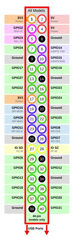
If you wish to use physical (BOARD) numbering you can specify the pin number as "BOARD11". If you are familiar with the wiringPi<sup>12</sup> pin numbers (another physical layout) you could use "WPI0" instead. Finally, you can specify pins as "header:number", e.g. "J8:11" meaning physical pin 11 on header J8 (the GPIO header on modern Pis). Hence, the following lines are all equivalent:
