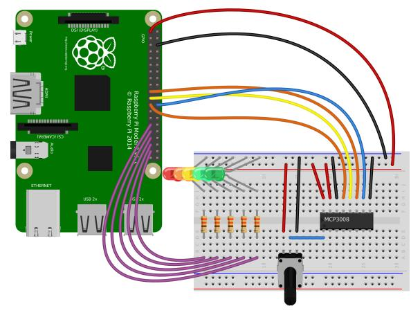
Continually print the value of a potentiometer (values between 0 and 1) connected to a MCP 3008 (page 149) analog to digital converter:
