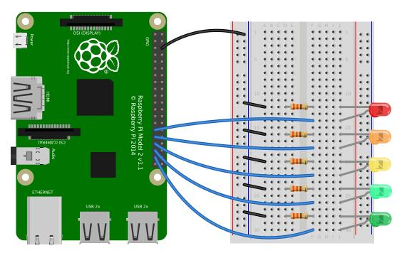
A collection of LEDs can be accessed using LEDBoard (page 157):
