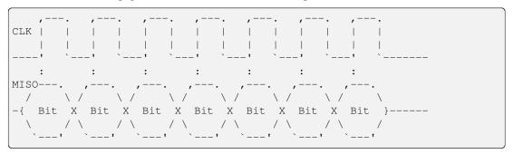
The following diagram indicates when data is read when <code>clock\_polarity</code> (page 231) is False<sup>881</sup>, but <code>clock\_phase</code> (page 231) is True<sup>882</sup>, equivalent to CPHA 1:
