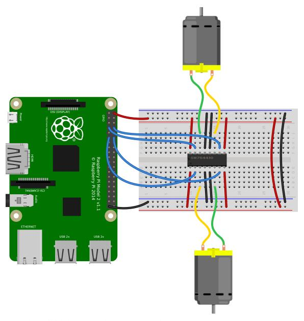
Use up/down/left/right keys to control a Robot (page 176):
