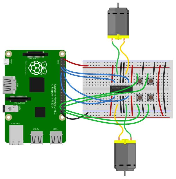
Use four GPIO buttons as forward/back/left/right controls for a Robot (page 176):
