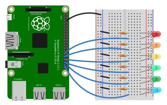
A collection of LEDs can be treated like a bar graph using LEDBarGraph (page 160):
