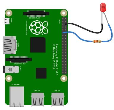
Any regular LED can have its brightness value set using PWM (pulse-width-modulation). In GPIO Zero, this can be achieved using PWMLED (page 127) using values between 0 and 1:
