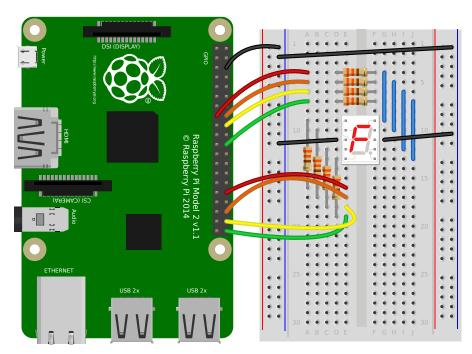
A common 7-segment display<sup>15</sup> can be used to represent a variety of characters using *LEDCharDisplay* (page 162) (which actually supports an arbitrary number of segments):
