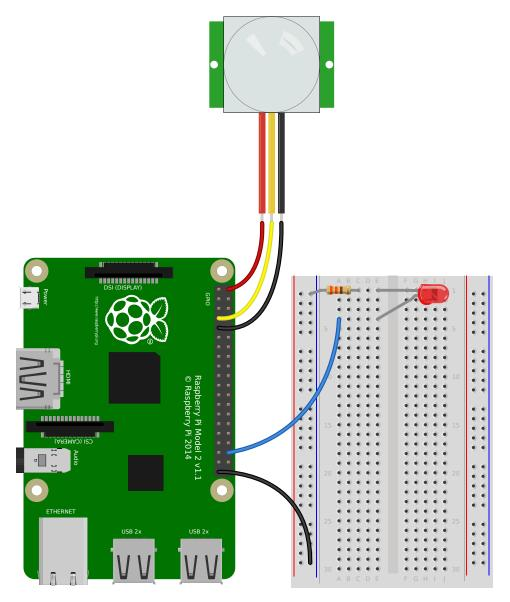
Light an LED (page 125) when a MotionSensor (page 109) detects motion:
