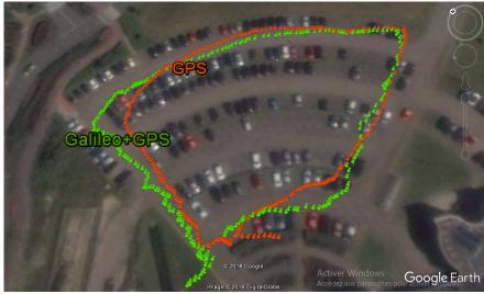
In the above figure the estimation of the trajectory that is based only on GPS does not follow too accurately the real pedestrian motion. However when both Galileo and GPS satellites are used together the position estimation is improved obtaining a pedestrian path closer to reality.
