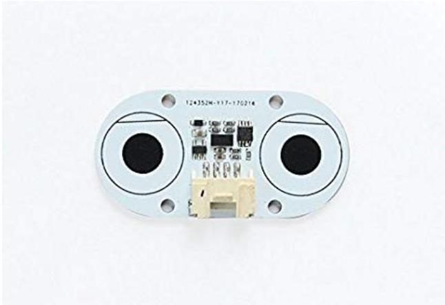
As you can see here, the [Distance Sensor](#) is the same sensor used on the [GoPiGo3](#) and on any DexterIndustries board that we support and that has a Grove port with an *I2C* interface on it.
