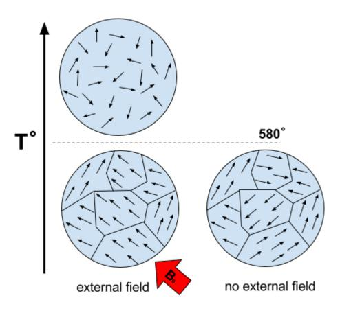
Magnetization is thus composed of two parts: (a) An induced portion  $(M_I)$  and (b) remanent portion  $(M_R)$ . The net magnetization is:
