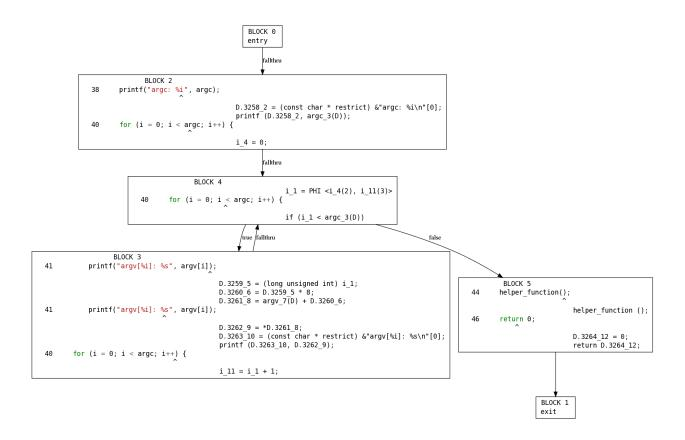
As is normal with SSA, GCC inserts fake functions known as "PHI" at the start of basic blocks where needed in order to merge the multiple possible values of a variable. You can see one in our example at the top of the loop in block 4:
