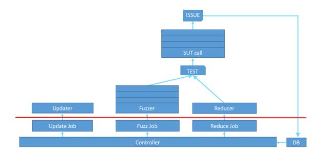
The red line represents an API boundary. Everything below it is part of the core infrastructure, while boxes above it are user-defined. However, you don't (necessarily) need to write a single line of code to describe your needs, since *Fuzzinator* can be configured through configuration *ini* files and it comes with several built-in building blocks that cover the most common scenarios and can be used out of the box.
