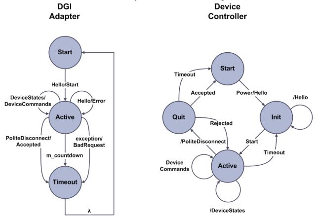
The protocol begins with both the DGI and the device controller in their respective start states. For the DGI, this state corresponds to some time after the DGI has created its TCP/IP socket that listens for connections from devices. For the device, the start state represents when the device is powered off or disconnected. First, the device powers on and
