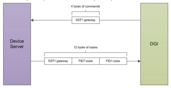
Both the command packet from the DGI and the state packet from the device server contain a stream of 4-byte floating point numbers. Other data formats such as boolean or string values cannot be used with the RTDS adapter; all the device states must be represented as floats. The command packet must contain every command for the devices attached to the server, while the state packet must contain every device state. It is not possible to send a subset of the commands,
