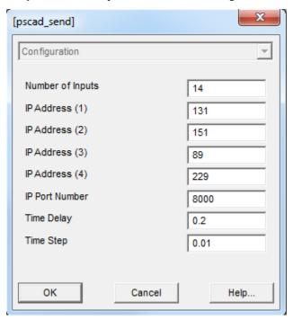
The number of inputs property should be set to the same value as that given for the *array\_merge* component, and should be the total amount of data points being sent out of PSCAD.
