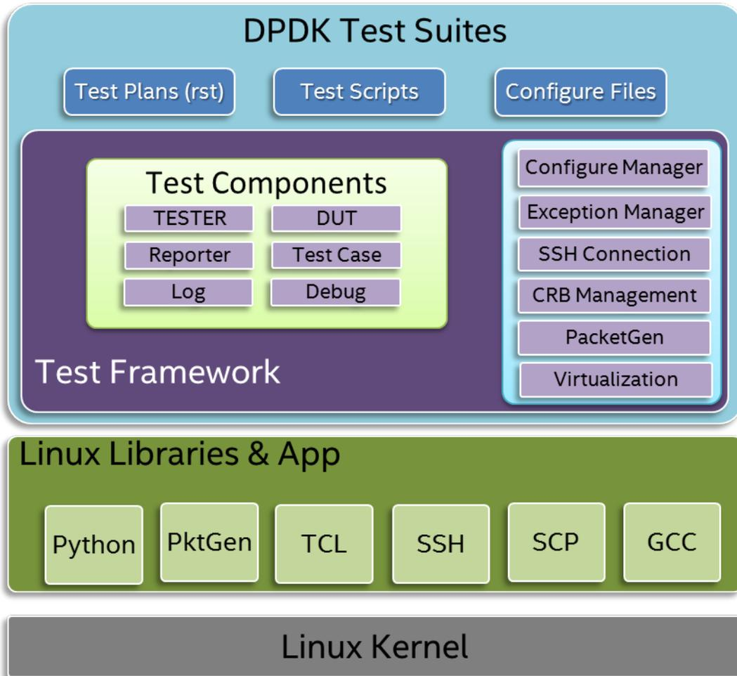
DPDK Test Suite environment includes DUT (Device under Test), Tester and packet generator. DPDK software will be deployed and run on DUT. DPDK Test Suite should run on the Tester.
