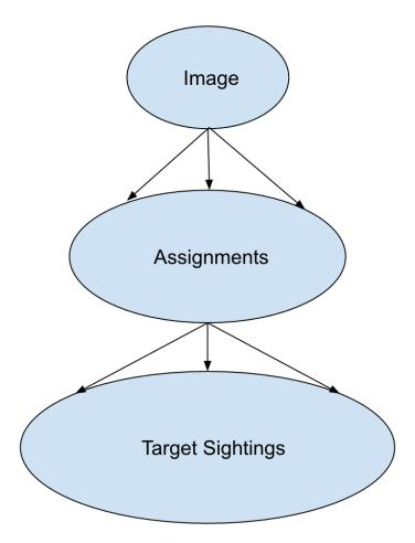
The above figure demonstrates the "one-to-many" relationships between the ground server abstractions. Each image has multiple assignments, which are distributed among various clients, and each assignment can have multiple target sightings.
