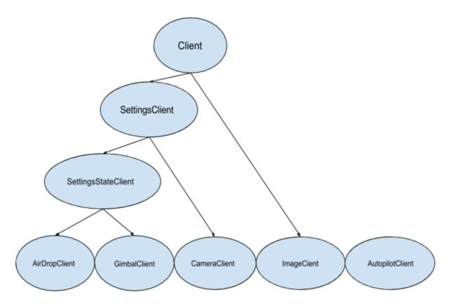
Client Class Diagram The Client abstraction simply defines a thread that continuously executes run().
