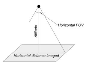
Horizontal distance imaged =  $2 \times altitude \times tan\left(\frac{FOV_H}{2}\right)$ Vertical distance imaged =  $2 \times altitude \times tan\left(\frac{FOV_V}{2}\right)$
