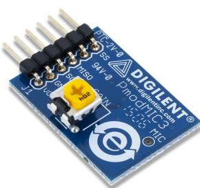
The Digilent Pmod MIC3 (Revision A) is small microphone module with a digital interface. With a Knowles Acoustics SPA2410LR5H-B MEMS microphone and Texas Instrument's ADCS7476 12-bit Analog-to-Digital Converter, you can capture your audio inputs with ease.
