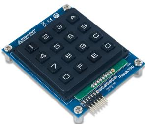
The Pmod KYPD is a 16-button keypad arranged in a hexidecimal format (0-F). By digitally driving a column line to a logic low level and digitally reading each of the rows, users can determine which button is currently pressed.
