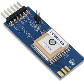
The Pmod GPS can provide satellite-positioning accuracy to any embedded system. By communicating through UART with the GlobalTop FGPM-MOPA6H GPS module, users may benefit from the 3-meter accuracy for any long term traveling.
