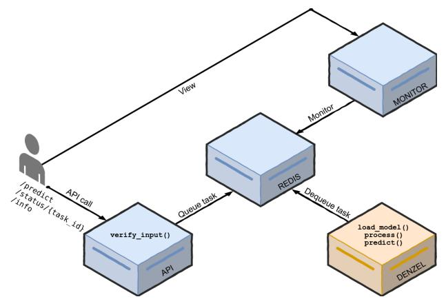
Fig. 1: High level overview of the denzel architecture. Each box is a container (API, Redis, denzel and Monitor). In orange is the main container, where the model will reside. On top of each container we can see the functions that will need to be implemented by the data scientist
