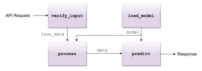
Fig. 1: API request flow through the four functions
