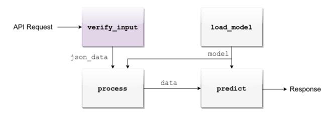
When a user makes a request, the first pipeline method that the request will meet is *verify\_input*. The *verify\_input* method is responsible for making sure the JSON data received matches the *interface we defined*. In order to do that, lets edit the *verify\_input* method to do just that:
