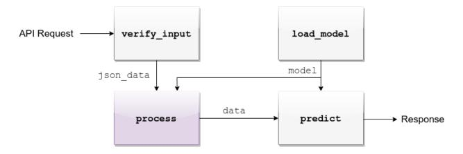
The output of the *verify\_input* and *load\_model* methods are the input to the *process* method.
