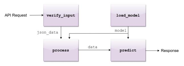
Fig. 2: API request flow through the four methods
