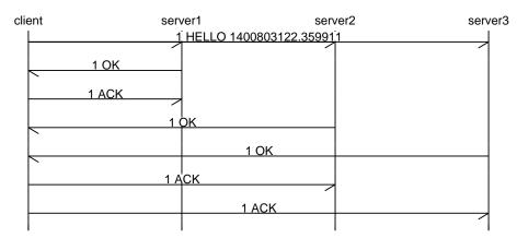
All messages are encoded as ASCII text. Command messages consist of a non-zero positive integer sequence number followed by a single space, followed by the command in capital letters, optionally followed by comma-separated parameters for the command. The following are all valid examples of command messages:
