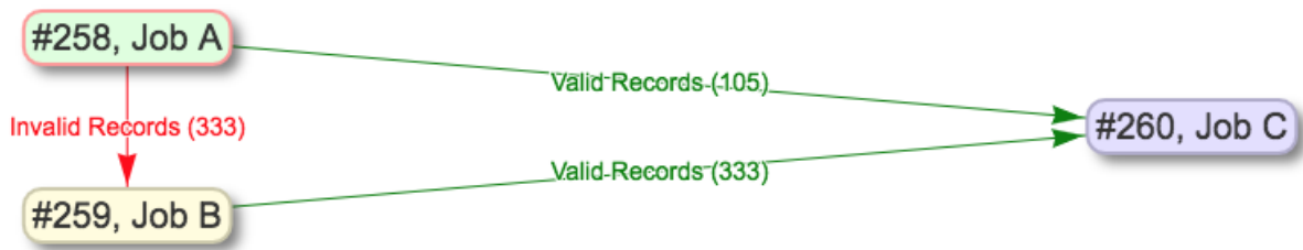
Fig. 45: Example of shunting Records based on validity, and eventually merging all valid Records
