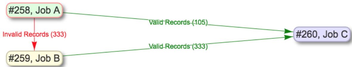
Fig. 81: Example of shunting Records based on validity, and eventually merging all valid Records
