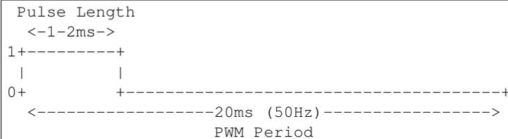
A duty cycle of 1ms will typically correspond to 0° rotation and a duty cycle of 2ms will typically correspond to 180° rotation. Although the precise values may differ depending on the type of servo.
