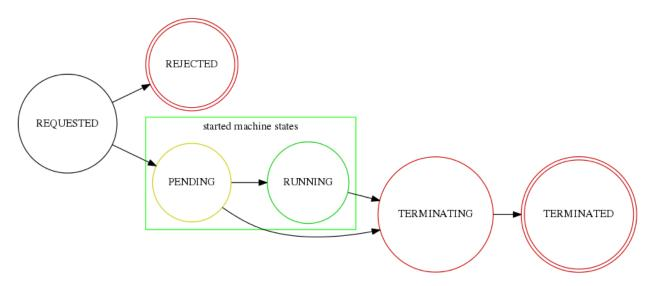
The PENDING and RUNNING states are said to be the *started machine states*. Machines in a started state are executing. However, just because a machine is executing doesn't necessarily mean that it is doing useful work. For example, it may have failed to properly boot, it may have crashed or encountered a fatal bug.
