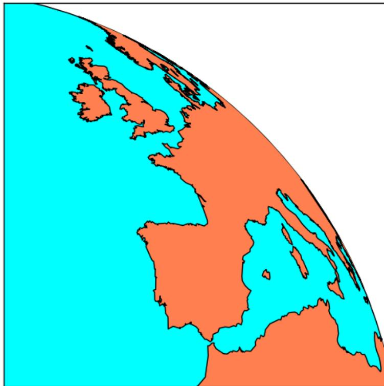
Some projections (the ones that look *like a satellite image*) accept setting the extension using the map coordinates. The projection parameters must be set (center point), and then the zone to show can be only a part of the globe.
