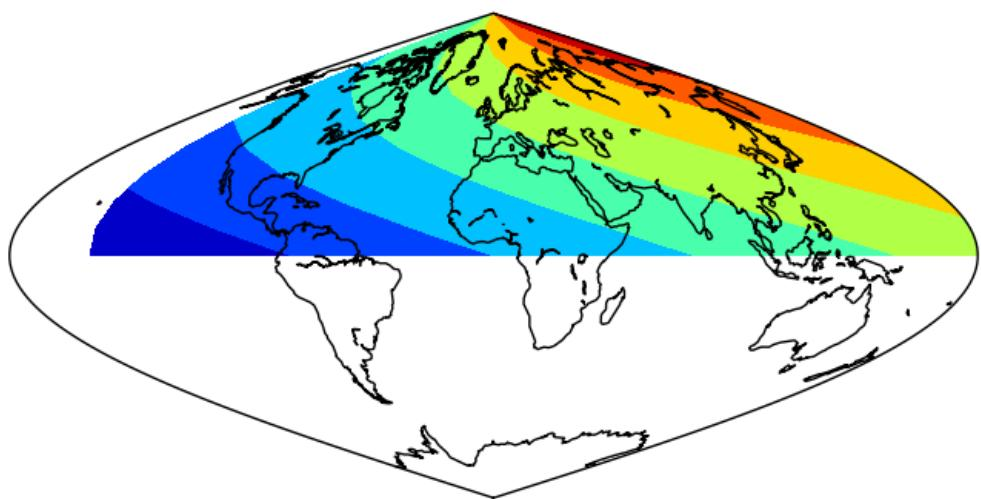
Fig. 2.8: The result without applying the method to the data array. Note that the blue (value 0) is not at longitude 0
