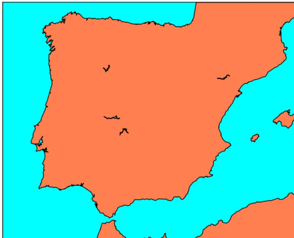
The lower-left and upper-right corners are passed as parameters, in longitude-latitude units, not in map units. This is the reason why in some projections fails, since a square in longitude-latitude may not give a good bounding box in the projected units.
