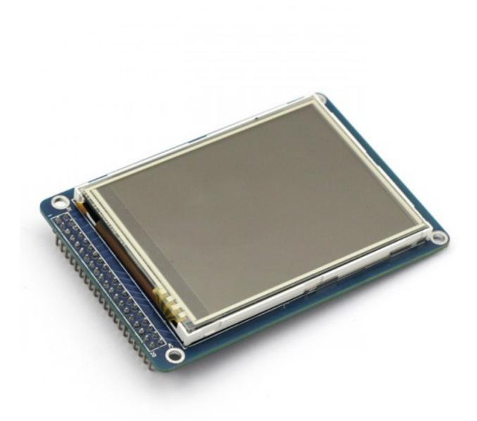
The SainSmart 3.2" TFT Touch screen is a LCD screen module with a SSD1289 controller. It also includes and SD card reader - however, this is not currently used by any of the functionality in the Aquarium Wise Controller.
