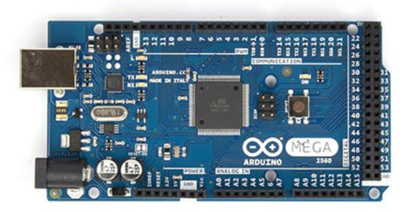
The Arduino Mega 2560 is a microcontroller board based on the ATmega2560. Although it is recommended that you purchase an official board from an Arduino reseller, there are many cheaper clones available that are suitable to use for the Aquarium Wise Controller.
