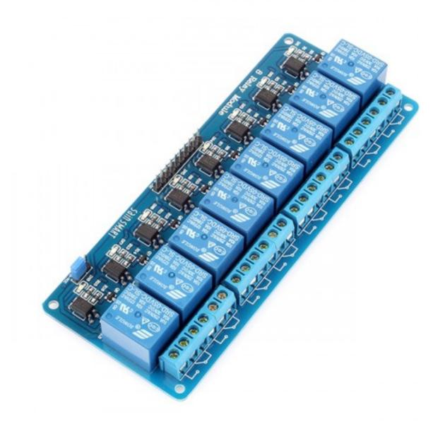
The SainSmart 8 Channel Relay Module is used to control the power outlets for lights, filters, heaters, etc.. Any relay board can be used in place of the SainSmart board - some software changes may be required depending on what signal the relay board is expecting (Some expect HIGH for off and others expect LOW for on).
