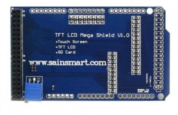
Although not required, the SainSmart TFT LCD Adjustable Shield makes the process of hooking up the 3.2" TFT to the Arduino much simpler. Some modifications are required if you wish to use it as a straight plug-in for the Arduino. These modifications are located further in to the documentation.
