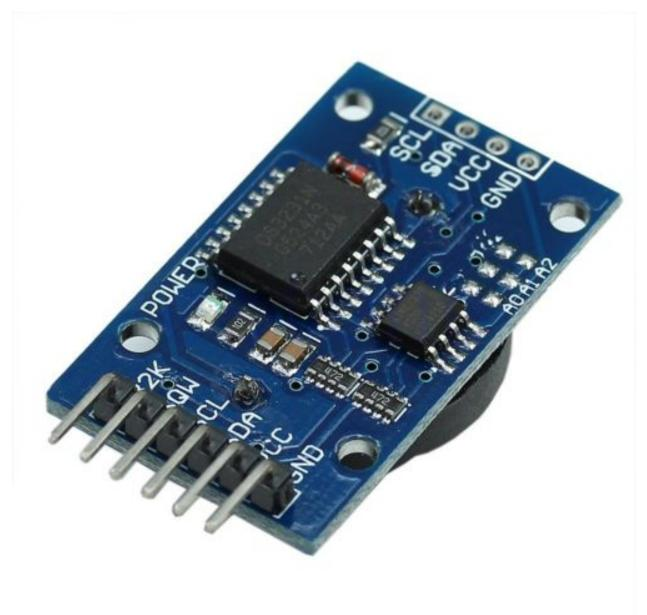
The DS3231 is a low-cost, extremely accurate I<sup>2</sup>C real-time clock (RTC) with an integrated temperature-compensated crystal oscillator (TCXO) and crystal.
