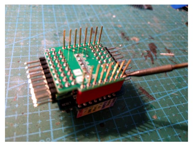
Next, connect your soldering iron, wait for it to get hot, and put it on one of the pins, so that it touches both the pin and the board.
