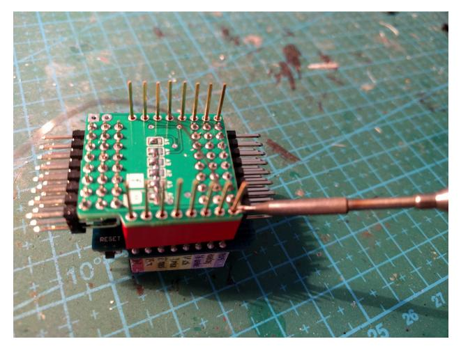
Wait a couple of seconds for the pin to get hot, and then touch the pin and the board with the solder wire. Let the solder flow into the hole around the pin. Then remove the solder wire and the soldering iron, and move to the next pin.
