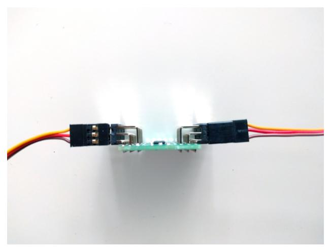
You can stack this shield with any other shields that either don't use the pins D1 and D2, or use them for  $I^2C$  and have a different address than set on this shield. If you want to stack more than one servo shield on the same board, you have to change their addresses with the jumpers on the back.
